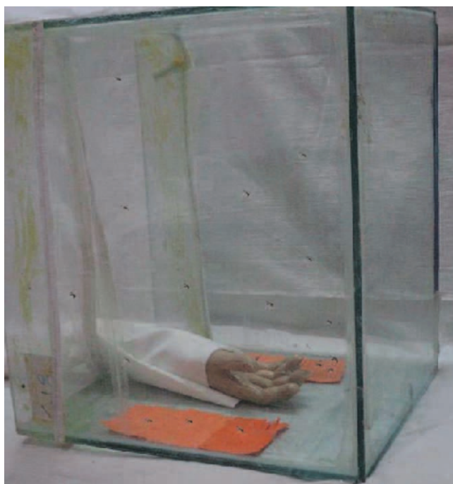
Figure 8 Insect-repellent testing cage. [Color figure can be viewed in the online issue, which is available at wileyonlinelibrary.com .]
